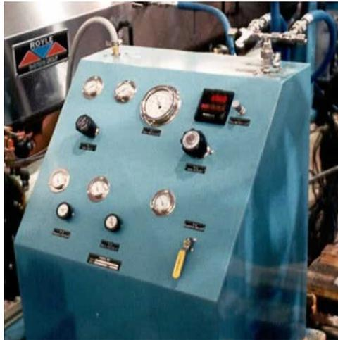
Royle's air-driven piston booster system integrates seamlessly with many nitrogen supply systems including bulk liquid or gas in addition to standard commercial gas cylinders. The system utilizes high accuracy non-pulsing regulators and stainless components and incorporates a
