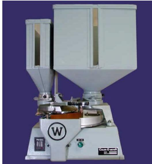
A Royle Color-O-Meter is designed for proportioning resin and one additive. The system comes complete with two hoppers and two rotating feed plates. The feed plates under each hopper rotate to meter the material from the hopper. The mixture ratio is controlled from a single calibration point.
