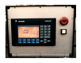
The process speed is adjustable with the touchscreen OIT which is mounted on a swing arm for easy operator access. The OIT has adjustable operating parameters that include process speed, ink tank air pressure, payoff and takeup tension, takeup pitch and inner/outer reel limits.
